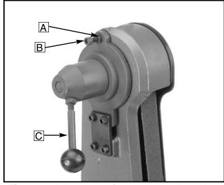
Figure 7. Adjustments for tension and tracking.
